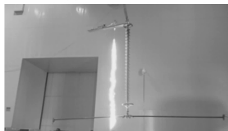
(c)电弧连通两极,间隙击穿
